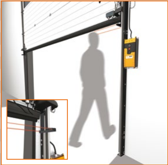
Predictive safety edge The predictive safety edge is located 8 cm ahead of the door. If the bottom of the door approaches an obstacle, a signal is immediately sent to the motor and the door stops and reopens. This means the safety edge works without coming into contact with people, goods or transport vehicles.
