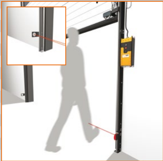
Stationary photoelectric safety sensor Motors with touch control must have a photoelectric safety sensor if the door opening is not visible to users while they are operating the door. There are two types: a model with a transmitter and reflector and a model with a transmitter and receiver. In both systems there is a transmitter attached to the rail on the control box
