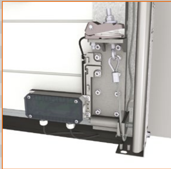
Slack cable device This safety device is installed on both hoisting cables and immediately disconnects the motor if one of the cables breaks or becomes slack.
