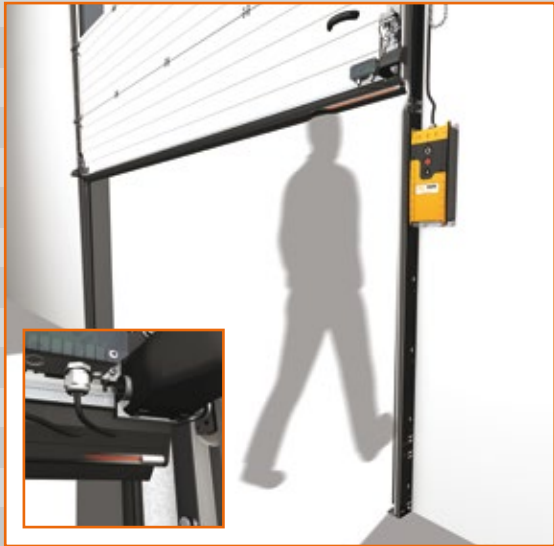
Standard safety edge The safety edge device is integrated together with a transmitter and receiver in the door's bottom rubber seal. If the signal is broken by an object or person, the door will stop and retract. The maximum contact pressure for the rubber seal is 40 kg. Choose the predictive obstacle safety edge if you have products that cannot withstand that level of pressure.
