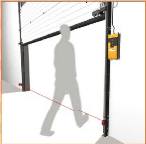
side and a reflector or receiver attached to the opposite rail. If the beam between the transmitter and the reflector/receiver is broken, a signal is sent to the motor to stop and reverse the movement. While the reflector system is sensitive to dust and moisture, this is not the case for the receiver model.
